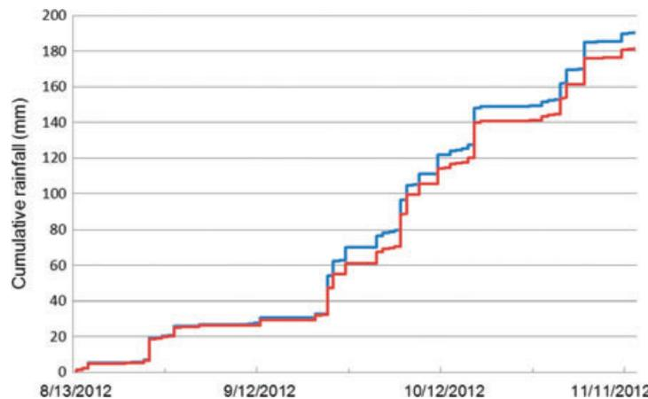
Figure 9. Cumulative rainfall recorded by the VP2 (blue) and the FO1 (red) station over the period 13 August to 12 November 2012, when located above a garage roof.
