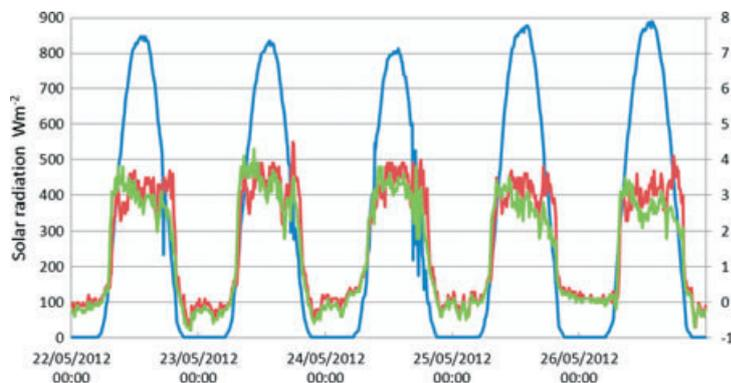
Figure 5. Solar radiation (blue, left-hand scale) and difference between VP2 and FO1 (red) and FO2 (green) temperatures (degC, right-hand scale), 22–26 May 2012.
