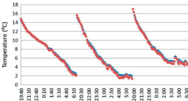
Figure 4. Rapidly falling temperatures measured by the VP2 (blue) and FO1 (red) stations on 26/27, 27/28 and 28/29 March 2012.
