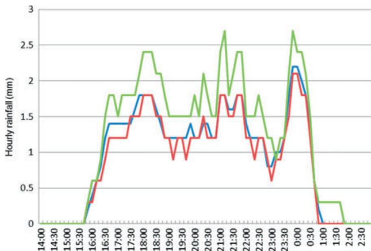
Figure 10. Running hourly total rainfall measured by the VP2 (blue), FO1 (red) and FO2 (green) rain gauges during a period of sustained rain on 12/13 July 2012.
