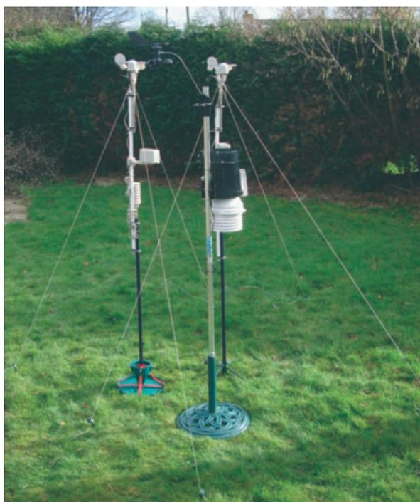
Figure 1. The VP2 weather station (centre) and the two FO stations on a garden lawn.
