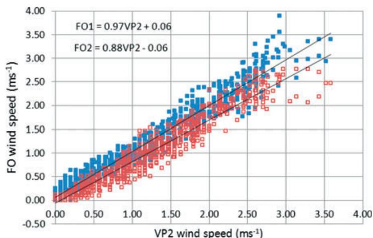
Figure 13. The relationship between hourly running-mean wind speed measured by the VP2 and the FO1 (blue) and FO2 (red) stations during the same period as in Figure 12.
