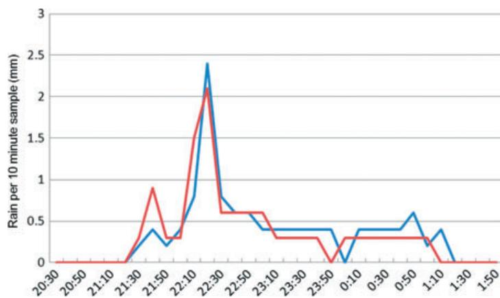
Figure 11. Rainfall per 10-minute sampling period measured by the VP2 (blue) and FO1 (red) rain gauges during a burst of heavy rainfall on 22 November 2012.
