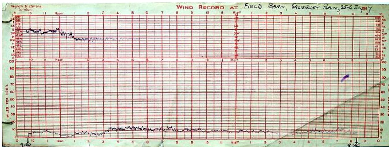
Figure 6. The first anemogram for Butler's Cross, dated 25-25 July 1917; unfortunately the ink ran dry – not an auspicious start! It is labelled as being for Field Barn, Chapperton Down, probably after the nearby Field Barn gun battery.
