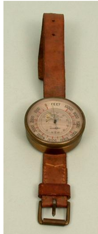
Figure 3: An example of a wristlet altimeter used by RFC pilots and observers; this version is graduated in 100s of feet to 10,000 feet.
