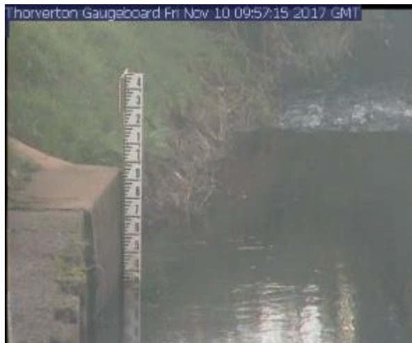
Stage board on the River Exe, monitored by webcam
