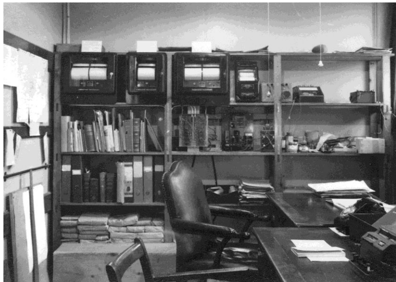
The office Mike Blackwell's and I shared. On the top shelf are chart recorders for solar and daylight radiation.
