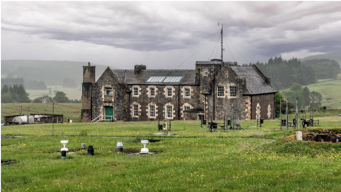
Eskdalemuir Observatory showing rain gauges and trials site. The Dines Pressure Tube anemometer can be seen on the roof of the building.
