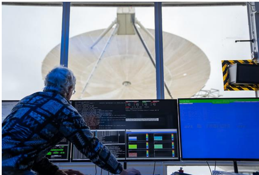
Figure 3 - The Chilbolton Advanced Meteorological Radar (CAMRa) and control room. The largest steerable meteorological radar in the world. The 25m antenna produces a very narrow beam (0.28 degrees), which is essential for probing turbulent processes in convective clouds. Picture courtesy National Centre for Atmospheric Science.
