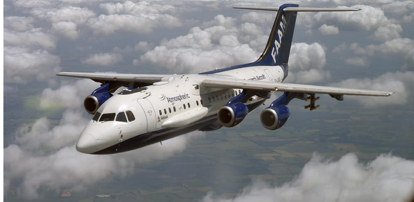
Figure 2 - A photograph of the FAAM Atmospheric Research Aircraft in flight. One turbulence probe is encased in the aircraft nose and another will be carried on one of the wings. https://www.faam.ac.uk/what-is-faam/ Picture courtesy National Centre for Atmospheric Science.
