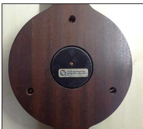
Reverse showing adjustment screw in centre
