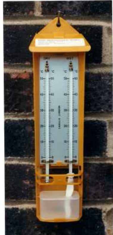
FIGURE 8 Humidity is measured most accurately with a wet- and dry- bulb thermometer
