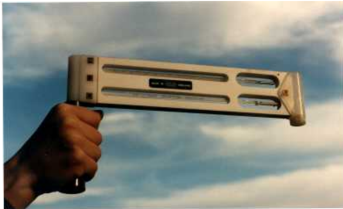
FIGURE 9 This type of wet- and dry- bulb thermometer is known as a whirling psychrometer
