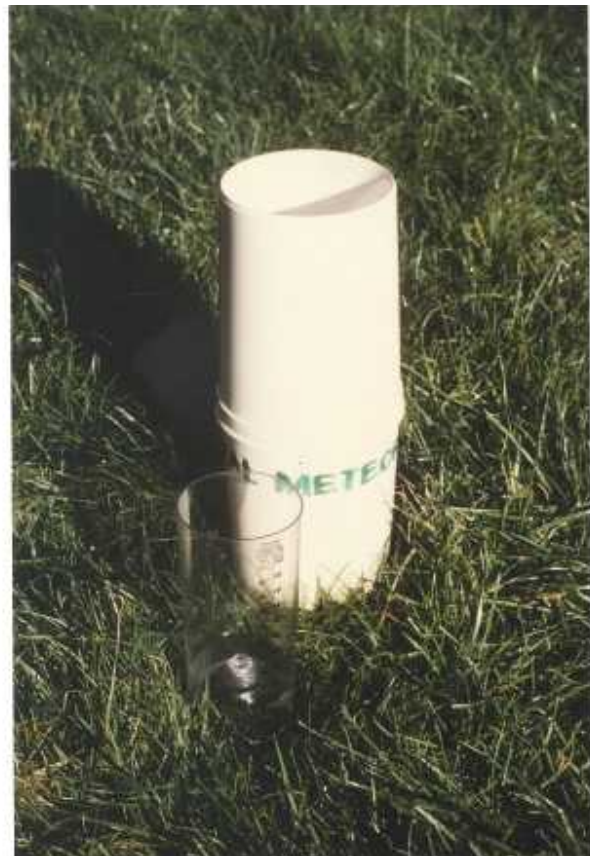
FIGURE 6 A cheap plastic rain-gauge with funnel and measuring cylinder
