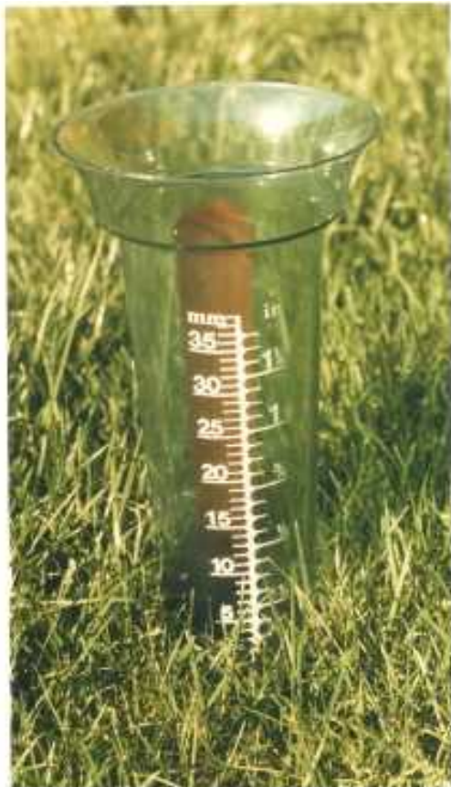
FIGURE 5 A simple plastic rain-gauge
